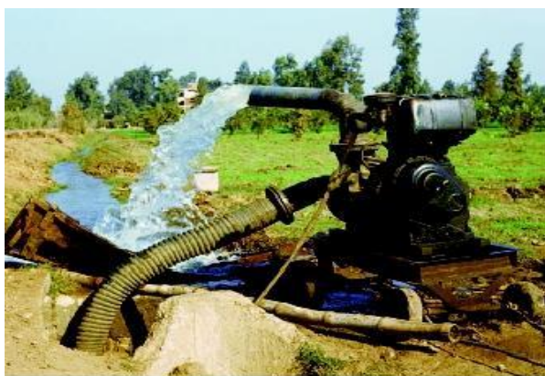
Figure 2: Diesel water pump for irrigation system used in Karangmojo
